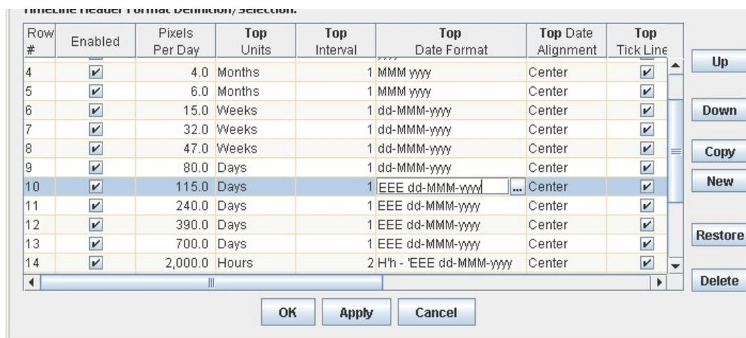
The “TimeLine” Format Dialog is used to format the headers for the Gantt and Schedule charts. It allows custom date formats, date alignment, alternating intervals to be defined for both top and bottom scales. This dialog is accessed from the chart headers by right clicking on the header and selecting “TimeLine Format...” from the pop up menu.
